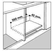
The panels of the adjacent cabinets must be made of heatresistant material. In particular, cabinets with a veneer exterior must be assembled with glues which can withstand temperatures of up to 100 °C.
